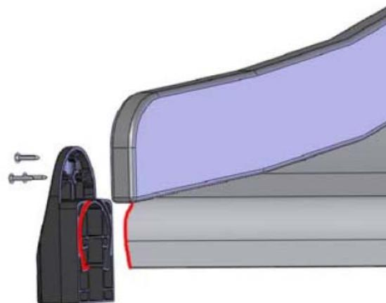
Insert sheet metal IN to the plastic cover.
