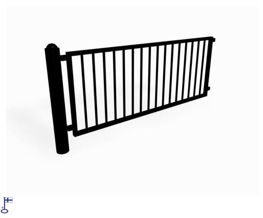
Fencing for greater enjoyment and safety. Flexible wrought iron fence with vertical square bars, one module height 900 mm and lenght 2000 mm. Complete sections (base section and extention sections) are affixed to the posts with a clamping ring and can therefore be turned to the desired angle. To create some differences in level, the sections may be stepped. Deep installation with wet concrete.
