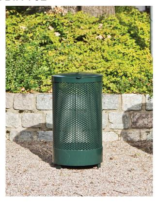
Large Joar litter has tight fitting lid giving cover against rain and animals. Material is durable 3mm perforated steel plate with four standard color powder coating. Free standing Joar has option to be fixed on hard ground with bolts or on soft soil with anchor and wet concrete. Chosen fixing accessory is included in delivery. Maintenance through hinged top lid by changing garbage bag.
