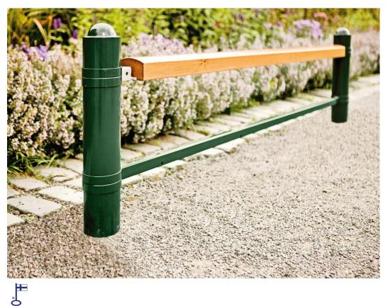
Flexible railing for train and bus stations. Steel railing with pine seating. With one mid-post, height 600 mm. The seating lintel and mid-posts are affixed using a clamping ring on the posts, and can therefore be positioned at any angle.
