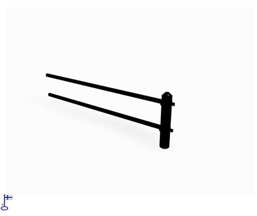
Extension section for railing NF9042. Single steel railing, 900 mm from the ground (c-c 2000 mm). The railing is affixed on the posts using a clamping ring and can therefore be angled as desired. Two bars in the middle.
