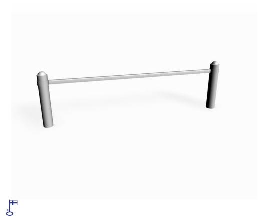
Flexible railing for public environments. Single steel railing, 600 mm from the ground (c-c 2000 mm). The railing is affixed on the posts using a clamping ring and can therefore be angled as desired. One bar in the middle.
