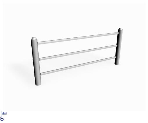
Flexible railing for public environments. Single steel railing, 900 mm from the ground (c-c 2000 mm). The railing is affixed on the posts using a clamping ring and can therefore be angled as desired. Three bars in the middle.
