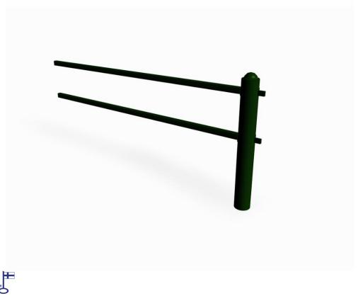
Extension section for railing NF9032. Single steel railing, 900 mm from the ground (c-c 2000 mm). The railing is affixed on the posts using a clamping ring and can therefore be angled as desired. Two bars in the middle.
