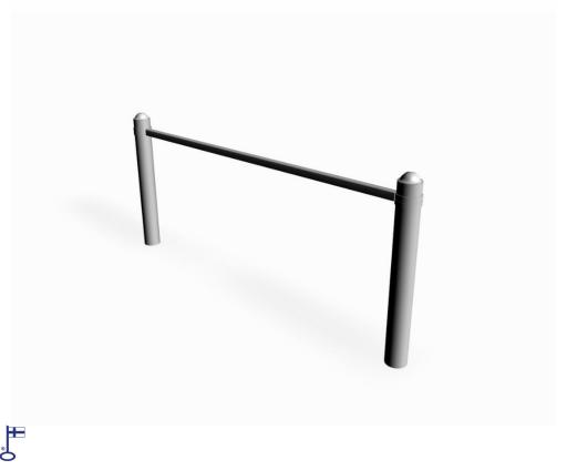
Flexible railing for public environments. Single steel railing, 900 mm from the ground (c-c 2000 mm). The railing is affixed on the posts using a clamping ring and can therefore be angled as desired.
