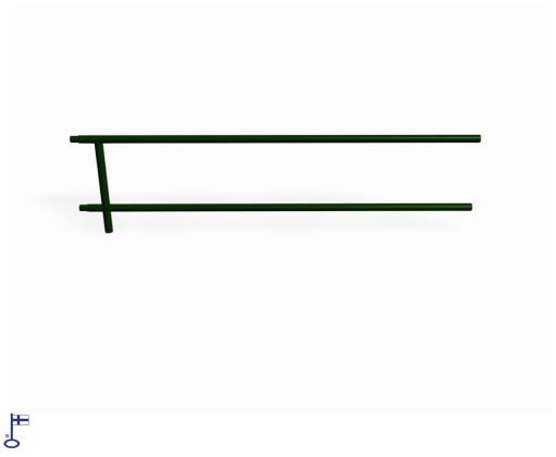
Extension section for railing NF7671A. Railing without seating plank; soft shapes in angled steel. With one mid-post 550 mm (c-c 2040 mm); designed for poured foundations. The images show the first sections.
