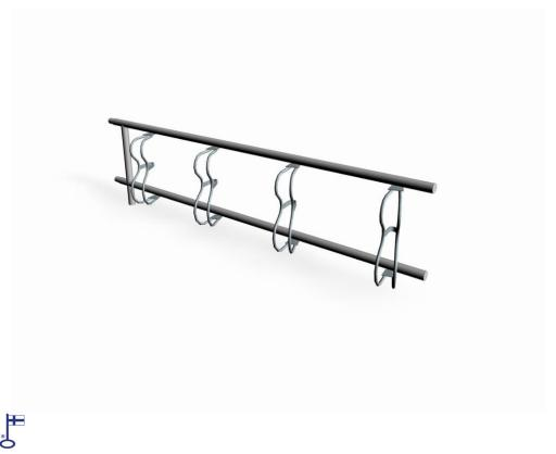
Urban is one sided bicycle rack for four bikes. The number of cycle spaces can be increased with extension sections or choosing the double-sided version. The rack is made of rounded angled steel with adjustable brackets. A frame mount RF7661M is available as an option.
