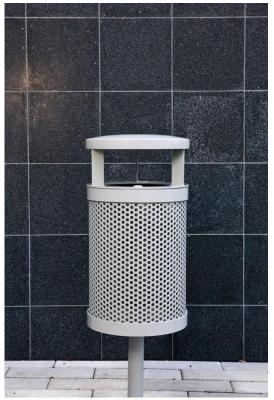
Litter-free playgrounds with Jakob. Jakob is a 35-litre litter bin. The litter bin has several fixing options - either set in poured foundations with a central post (50 mm), wall-mounted using a bracket for wall mounting (NF2472), or installed using a bracket on an existing post (105-120 mm) (NF2473). Jakob is made from 3 mm powder-coated steel.
