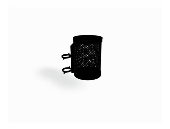
Litter bin with lid. Reuben is a litter bin made from 3 mm powder-coated steel, and has a tight-fitting lid. The bin has a volume of 35 litres and can either have poured foundations with a central post (40 mm) (NF2465), or be fixed to the wall (NF2466) or fitted on an existing post (105-120 mm).
