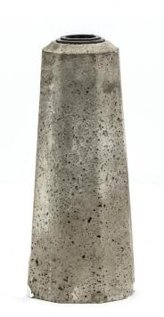
Underground concrete foundation for 60mm diameter post. Concrete foundation is sinked into 500mm deep pit and then covered with soil and compressed carefully.
