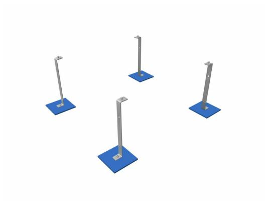
Anchorage component for free standing Park furniture like benches, tables and bicycle racks. Dig about 50 cm deep hole and put the anchor plate to bottom. Screw the metal frame to the plate and other end to the furniture leg. Then cover the hole and compress it. The Foundation set includes four anchoring plates and metal frames.
