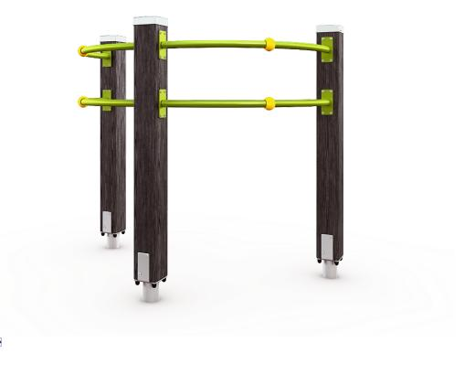
Fitness equipment intended for seniors, consisting of three upright posts and four curved metal bars, each holding a movable ball. The total height is 1,305 mm. The idea is to move the balls along the bar. The curved motion can be used to rotate the shoulders and open the chest. Highly effective stretching device when used from the outside. Provides exercise for the chest, elbows and shoulders.
