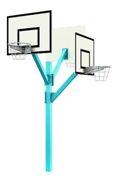
A basketball stand with three baskets. The baskets can be raised and lowered and can also be rotated on the pole during assembly. The sock and the ring of basketball hoops are stainless steel. Boarding of the basketball hoop is 21 mm painted plywood.
