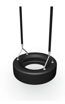
The length of the chains is about 160 cm. The swing seat is suitable for the following swings: 220001M, 220002M, 137414M, 137412M, 137418M, 175074, 175075, 220061M and 230050. The material of the chains is polished austenitic stainless steel, 6 mm thick. The chains have plastic coatings that protect the child. The seat is made of rubber.
