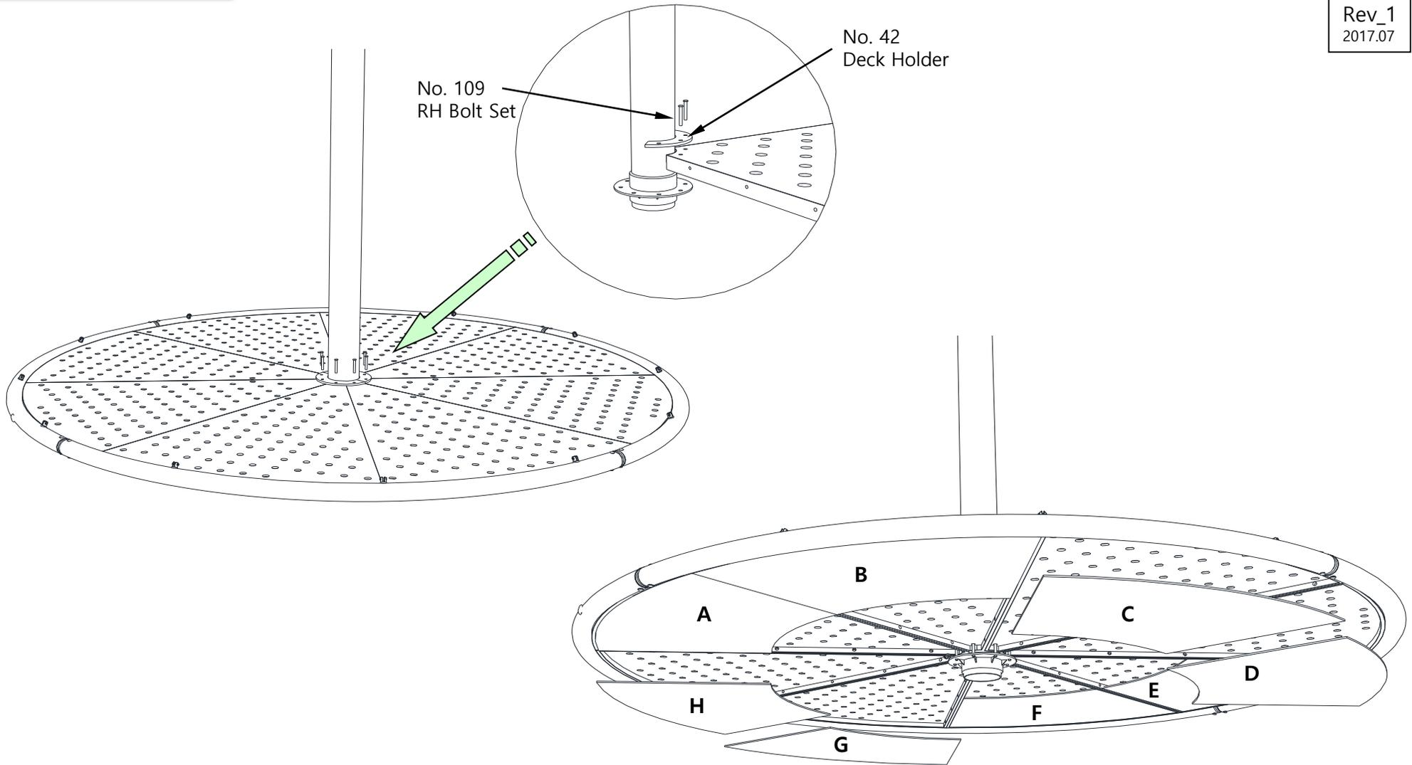
**Assemble Deck Cover Plate like C,D,G and H after assembling decks**
